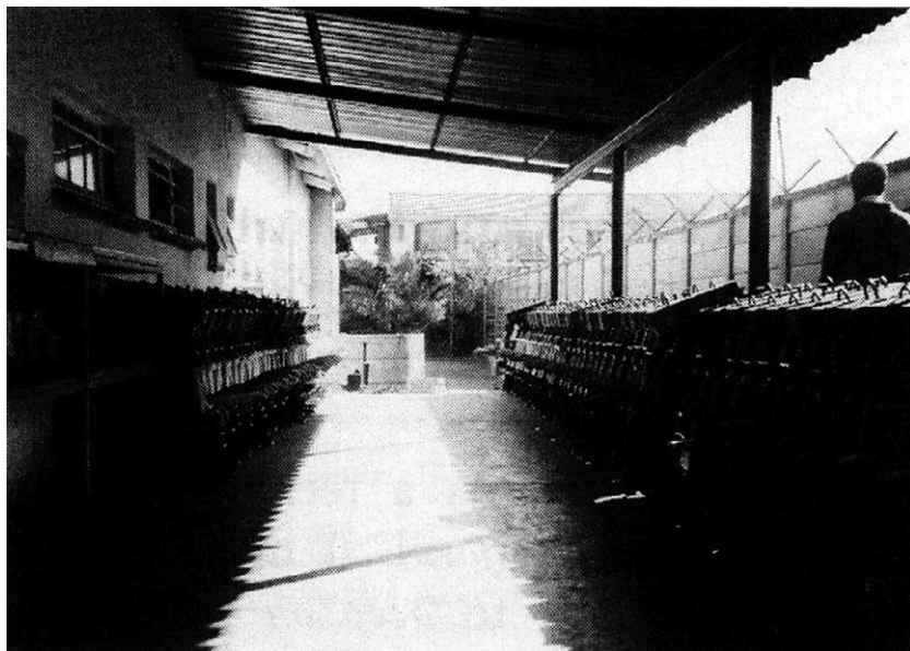
Figura 4. Hilera de bombas Bush en V&W Engineering
